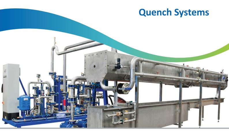
Denco Fluid Systems offer both quench spray / flood bath systems and quench tank systems. These are used commonly in metal process industries including wire extrusion. The systems are designed based on production flow rates, product properties and product temperatures.
